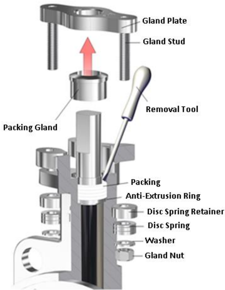
FIGURE 8. UPPER STEM PACKING REPLACEMENT
