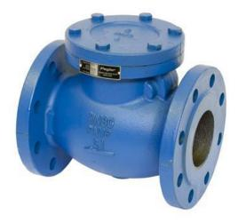
The Pegler type V914 Valves are Cast Iron swing check valves which are intended to prevent back flow in sections of pipe work and equipment an provide a long trouble-free service, it is intended to be used in the horizontal position however I can be used in a vertical pipeline. They are used for high velocity liquid services to prevent a change to the direction of flow caused by back flow and are available in sizes DN65 to DN300.
