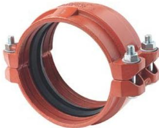
The *Shurjoint* Model H305 HDPE couplings feature four bolt housings and a series of sharply machined teeth which positively grip the pipe as the coupling bolts and nuts are tightened. The result is a leak-tight joint that is as strong, or stronger than the pipe itself. The H305 also features a contoured housing with integral ramps along the outside diameter to help the coupling slide over most obstacles during the relocation of pipe runs.
