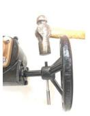
13. Following step 12, tighten the bolt on the left and loosen it by quarter turn. Make sure the valve disk is rotatable, then tighten the nut.
