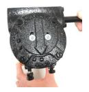
17. Secure the pin by hammering it in.
