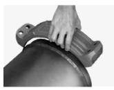
After welding use an R-88 housing segment as a gauge to check the weld size by ensuring full and smooth engagement. The housing ring pocket must fully engage the ring without interference from the weld fillet material.
