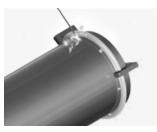
First, weld the butt ends of the ring together. Next, tack weld the ring onto the pipe at several locations. Remove the ring clamps or other positioning devices.
