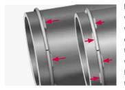
For lower pressure applications, weld rings need not be fully welded around the entire circumference of the pipe. in this case, partial ring welding will provide sufficient strength. In case of partial ring welding, the weld shall be processed on
