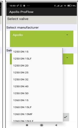
After clicking on the blue **Select Type** line, the list of valves of the given manufacturer will open. Select the required valve type. For simpler orientation and selection, also the picture for each valve type will be displayed for you.
